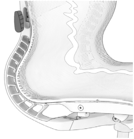
17.1 Remove No Arm Plug from opening in Beam.
