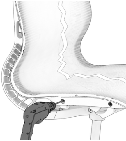
19.1 Using a Power Driver with a T-27 bit, remove Shoulder Bolts.
