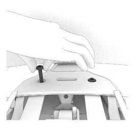
27. Using T-40 torx remove 2 screws from tilt assembly.
