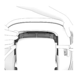
14. Lay chair on back. Using flat head screw driver pry away (both sides until seat lock bar comes out).
