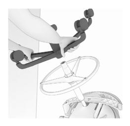
2. Disengage the base from cylinder.
