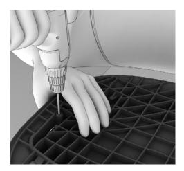
3. Using a power driver with a T-20 torx bit remove screws in seat pan.
