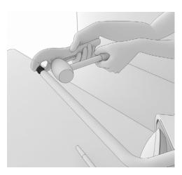
9. Clamp on to a glide using a vice grip and tap vice grip using a rubber mallet until glide comes out. Repeat the step on other legs to remove the remaining 3 glides.
