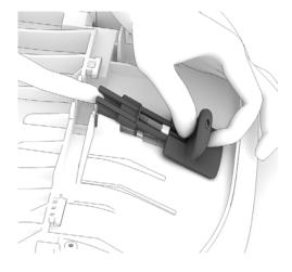
20. Slide latch to outside of seat frame until tabs are disengaged.
