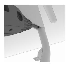
5. Using a power driver with a T-15 torx bit remove arm screws from back side.
