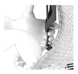
46. Using a nose plier remove hook on the bottom of the lumbar assembly.
