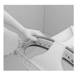
31. Turn it over and remove back attachment screws using a T-20 torx.
