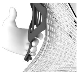
47. After disassembling one side, pull the bow back so that it does not engage again.
