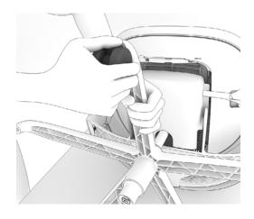
1. Hold base and pull hard to remove caster from base.
