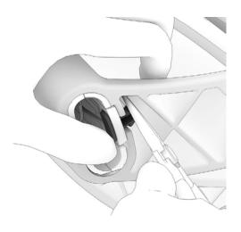
8. Using nose plier depress the retention clip.
