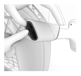
10. Depress the lock inward and pull the arm up to remove.
