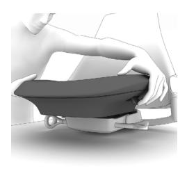
16. Release the seat lock move seat to the backward position.
