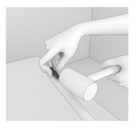
10. Place a rigid spacer between wheels on the body of caster and tap on it with a rubber mallet until caster wheel assembly comes off. Repeat the step on other legs to remove the remaining 3 casters.
