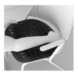
4. Slide seat pan rearward until all tabs are disengaged.
