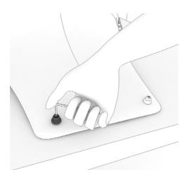
37. Use a T-20 torx wrench remove 1 screw from each pivot joint.
