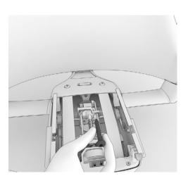
25. Remove the bolt from tilt assembly.
