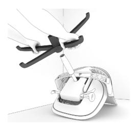
4. Disengage the base from cylinder.
