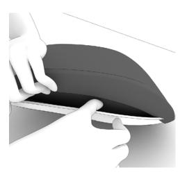
23. Remove the seat foam from the seat bottom.
