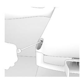
30. Remove top screws from each side using a T-25 torx from the frame.
