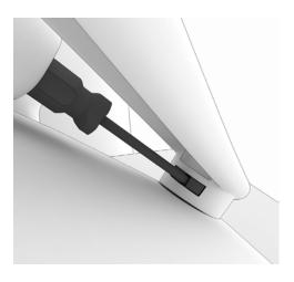
35. Insert a screw driver and rotate to expand the clip.
