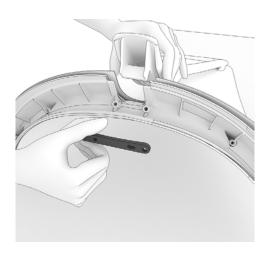
34. Using hand slightly pull back the spine from the back and remove the spine bracket plate from bottom of the back.
