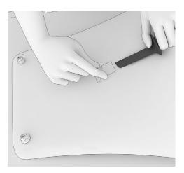
41. Using thumb & fore finger squeeze handle snaps together.
