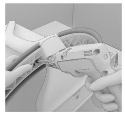
32. Remove back attachment screws using a T-40 torx.
