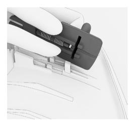
21. Unsnap the latch from seat frame and remove spring.
