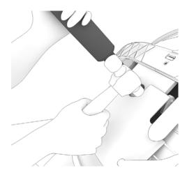
5. Place one hand on can of cylinder and hit with hammer.
