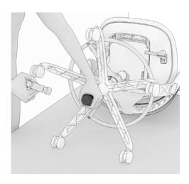
1. Place nylon cap over the end of cylinder and strike with hammer.
