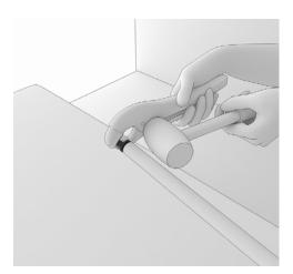
11. Clamp on to a caster receptacle using a vice grip and tap vice grip using a rubber mallet until receptacle comes out.
