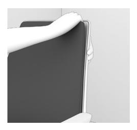
12. Carefully slide fingers between front fabric cover and frame, pull firmly. Pull corners first and then center.
