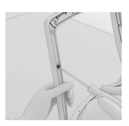
16. Using a phillip head screw driver remove all screws from retainer.
