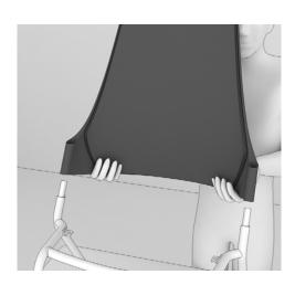
8. Pull or tap upward to remove back.
