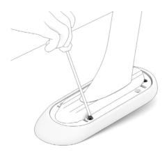
12. Using T-20 torx driver remove arm pad screws (4 screws for adjustable pad, 1 screw for fixed pad.
