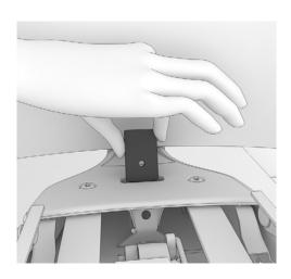
26. Remove the plate from the tilt assembly.
