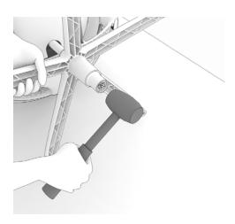
3. Hold base legs firmly and strike the bottom of cylinder with a rubber mallet until base comes loose.
