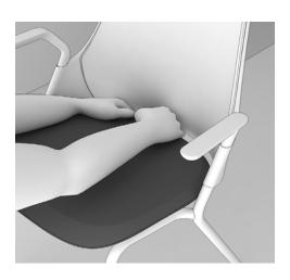
2. Pull up on rear of cushion to disengage snap and slide seat cushion forward.
