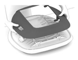
19. Remove seat skirt. Seat skirt is also held on by 4 clips. Carefully pull the seat skirt loose from these clips. With screw driver pry out and remove any clips that remain lodged in the seat frame.
