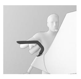
6. Using a rubber mallet tap on bottom of arm until arm comes out.
