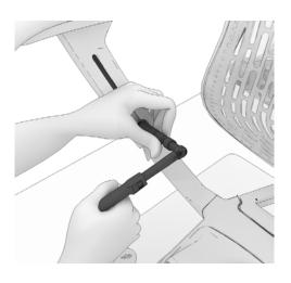
13. Using 13mm deep socket remove the post.
