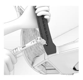
18. Use 4" T30 torx bit to remove the arm casting from tilt assembly.
