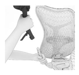
17. Slide the entire assembly up to remove the arm.
