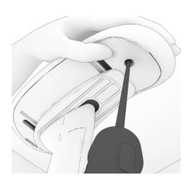
20. Using philips T20 torx bit remove the front of the arm pad bolt.
