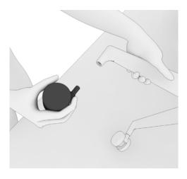
50. Pull straight out to remove the caster. Repeat the same to remove other 4 casters from base.
