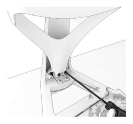
34. Using T25 torx screw driver remove the screws.
