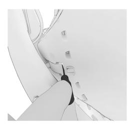
3. Slide the flat head screw driver into the slot and depress the spring clip.
