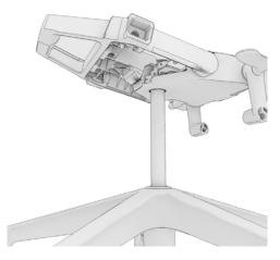
43. Bottom tilt cover removed from the tilt assembly.
