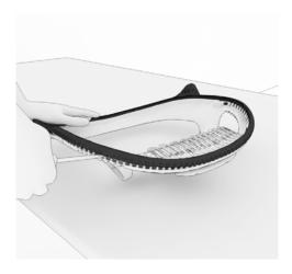
9. Using flat blade screw driver pry up gently to remove seat ring.
