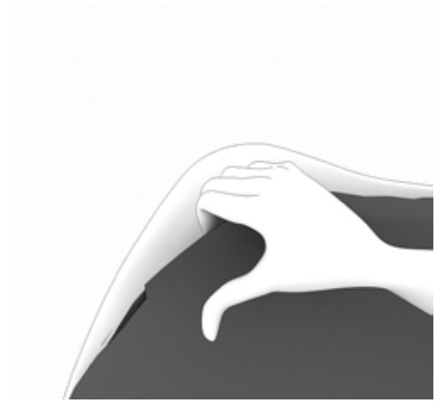
46. Remove the fabric from seat.
