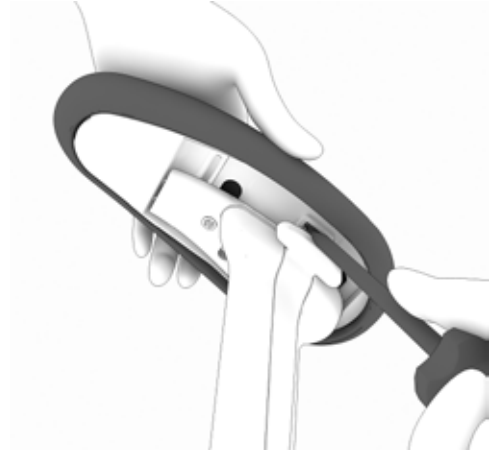
27. Slide arm pad to outermost position and insert straight head screwdriver against inside of retainer clip. Pry clip outward while lifting up on arm pad.
